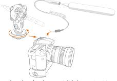
When using the shockmount, it is important to cross the rubber band on both sides (diagram below). This will secure the iShotgun in place and help minimise handling noise.
